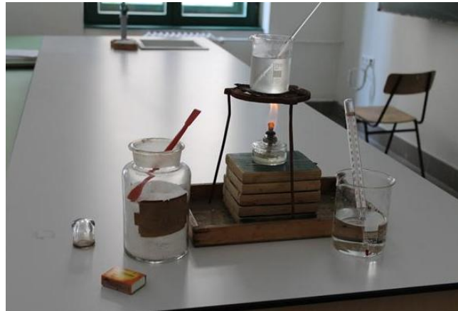
Picture 1 Measuring set for boiling point determination
